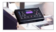
CAPACITIVE TOUCH SCREEN Ergonomic touch screen with all critical functions on display.
